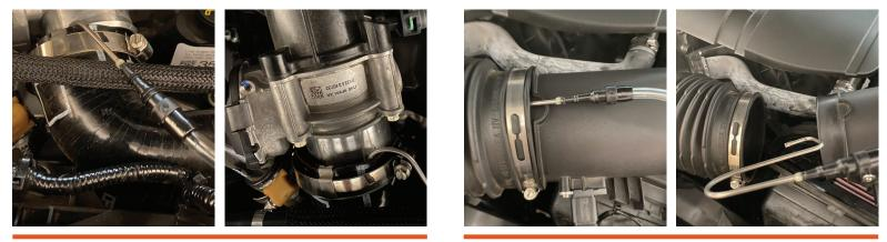
**BEST** (INTAKE HOSE AT ENGINE THROTTLE BODY)
